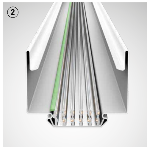
11-core current conducting profile 5 \times 2.5 \text{ mm}^2 + 6 \times 1.5 \text{ mm}^2 3 separate circuits 2 control lines for DALI signal 2 independent emergency light circuits
