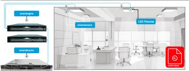
The smartdirector provides a browser based user interface for all of the smartengine devices, stores smartsensor data and provides web services and BACnet/IP APIs.
